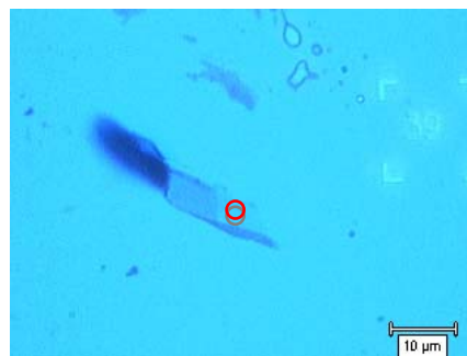
Fig. 1. An optical image of a candidate graphene flake. The circle shows the location of the laser spot used to obtain the Raman spectrum in Fig. 2.
