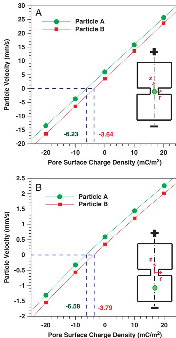
**Figure 4.** Particle velocity (A) at the center of the pore and (B) 200 nm away from the pore as a function of membrane surface charge density. All other simulation conditions are the same as in Fig. 2.
