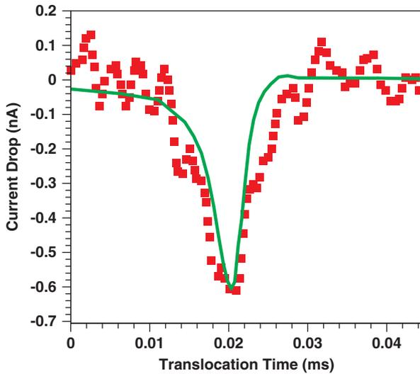
**Figure 2.** Ionic current drop generated in the system by a 30 nm spherical particle with a surface charge density  $-22 \text{ mC/m}^2$  passing through the nanopore. Here  $\sigma_m = -15 \text{ mC/m}^2$ ,  $E = 1 \text{ mm}$ ,  $F = 5 \text{ mm}$ ,  $H = 600 \text{ nm}$ ,  $W = 1200 \text{ nm}$ ,  $h = 50 \text{ nm}$ ,  $e = 75 \text{ nm}$  and  $C_0 = 0.2 \text{ M}$ . The solid line and symbols correspond to numerical simulation and experimental results, respectively.
