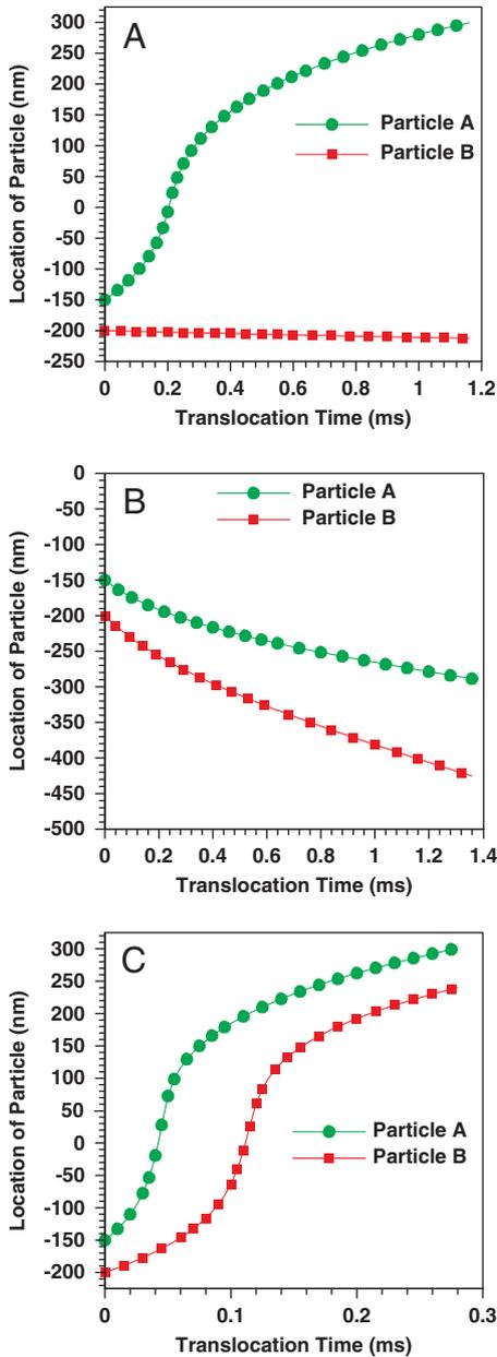
**Figure 5.** Trajectories of Particle A and Particle B with time for a membrane with a surface charge density of (A)  $-4.0 \text{ mC/m}^2$ , (B)  $-8.0 \text{ mC/m}^2$ , and (C)  $4.0 \text{ mC/m}^2$ . Particles are initially 50 nm apart. All other simulation conditions are the same as in Fig. 2.
