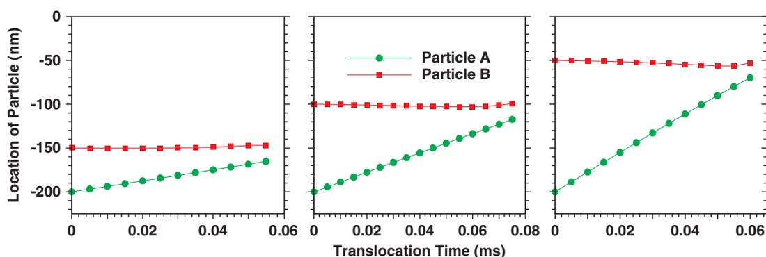
**Figure 7.** Trajectories of Particle A and Particle B with an initial separation distance (left) 50 nm, (middle) 100 nm, and (right) 150 nm for a pore surface charge density  $\sigma_m = -4.0 \text{ mC/m}^2$ . All other simulation conditions are the same as in Fig. 2.
