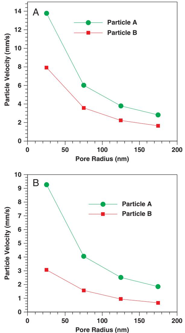
**Figure 3.** Particle velocity (A) across an uncharged membrane ( $\sigma_m = 0.0 \text{ mC/m}^2$ ) and (B) across a membrane with surface charge density  $\sigma_m = -2.0 \text{ mC/m}^2$  as a function of pore radius. Particle A: 10 nm diameter and  $-7.0 \text{ mC/m}^2$  surface charge and Particle B: 30 nm diameter and  $-3.3 \text{ mC/m}^2$  surface charge. All other simulation conditions are the same as in Fig. 2.
