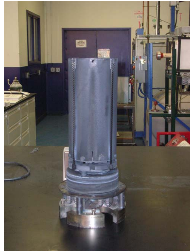
Graphite furnace used for HIPing
